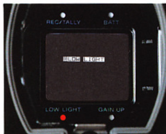
The light is insufficient. Add more light or raise the video output level via the gain selector.
