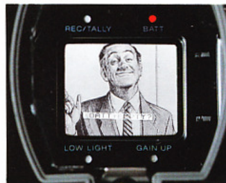
The battery voltage is below approx. 11.0V. Replace the battery with a fully charged one.
