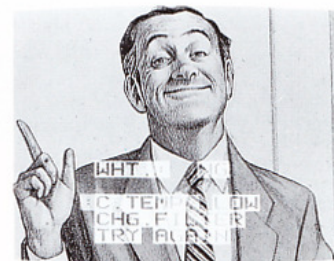
The color temperature is out of automatic control range. Change the filter and repeat the balancing procedure.
