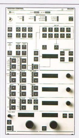
allowing immediate, non-sequential access to individual function groups such as registration, centring, shading, video, timing and optics.
