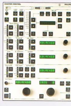
In addition, manual modifications of set-up data (e.g. bias light, RGB beams, shading, etc.) are indicated by an extensive LED display.
